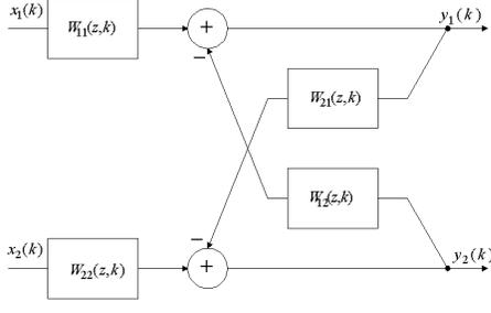
**Figure 2.** Feedback separation network
