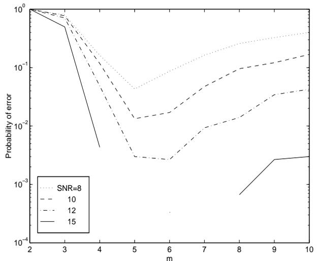
Figure 2: Probability of error as a function of  $m$ , the number of columns of the data matrix ( $N = 25$ ,  $\alpha = 0.01$ ).
