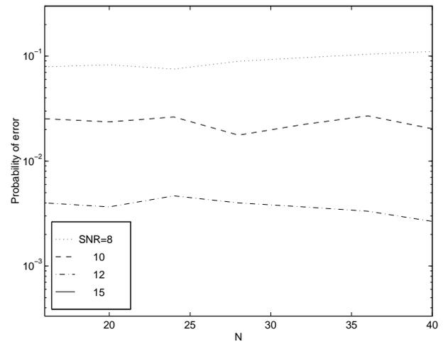
Figure 1: Probability of error as a function of the number of data points  $N$  ( $\alpha = 0.01$ ,  $m = 6$ ).
